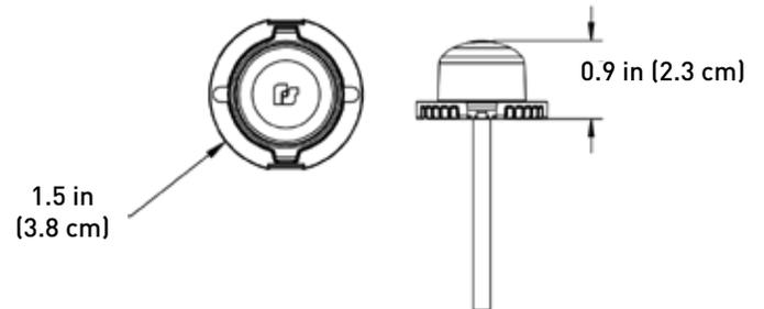
For best performance at peak intensity, it is recommended to keep the Federal Signal logo horizontal to the ground as shown above.
