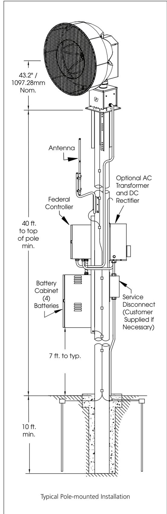
Typical Pole-mounted Installation
