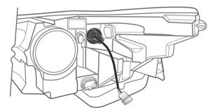
When the base stops in its rotation, pull it out of the socket. 2
