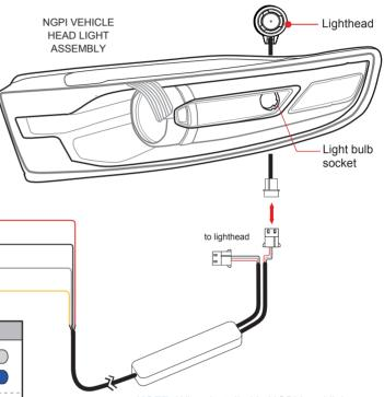
**NOTE:** When installed in NGPI head light assembly, the light projects towards the 45 degree angle for superior intersection warning.
