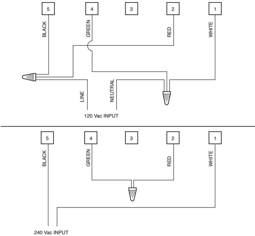
Figure 4 PS600 Wiring schematic
