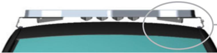
Image of Valor light bar on Dodge® Charger with standard “Hook mount”
