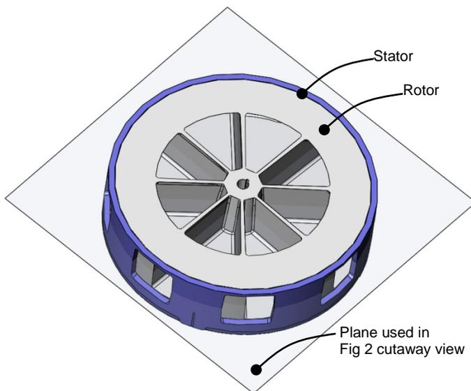
Fig 1: Rotor and stator in a typical electromechanical siren
