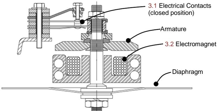
Fig 3: Electromechanical horn mechanism in an unpowered state
