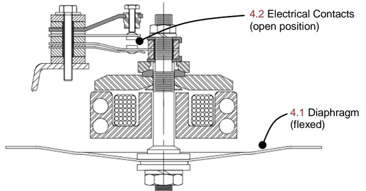
Fig 4: Electromechanical horn mechanism in a powered state (armature has reached lower travel limit)
