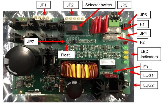
Figure 3 Position of fuses and connectors on charger assembly PCB (2005305)
