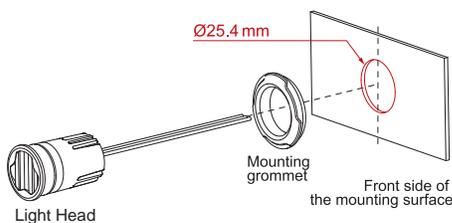
2. From the front, install the appropriate mounting grommet\* onto the cutout and insert the light head.
