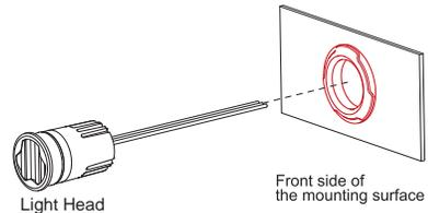
3. Ensure that the optical stripes are aligned vertically.
