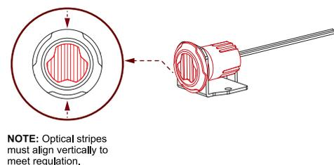
\*Two mounting grommets are included for various material thicknesses.
