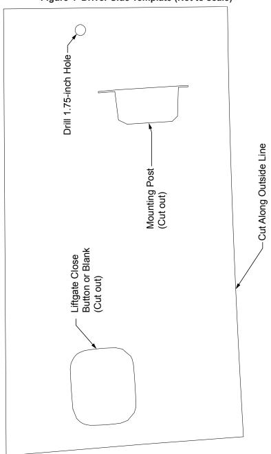
Figure 4 Driver Side Template (Not to scale)
