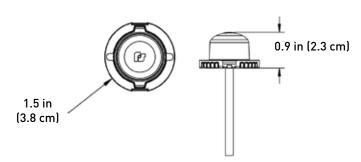
For best performance at peak intensity, it is recommended to keep the Federal Signal logo horizontal to the ground as shown above.
