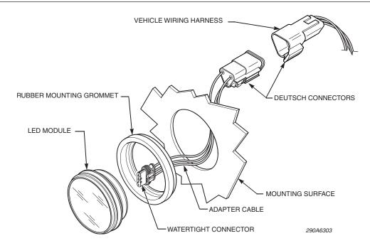
Figure 1: Connection between LED module and vehicle wiring harness
