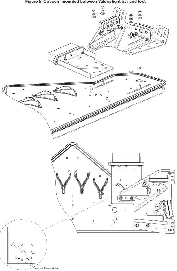
Figure 5 Opticom mounted between Valor® light bar and foot
