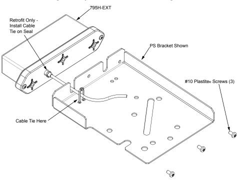
Figure 2 Opticom secured in mounting bracket
