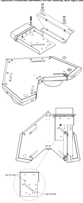
Figure 7 Opticom mounted between 3-Pod Vision® SLR light bar and foot
