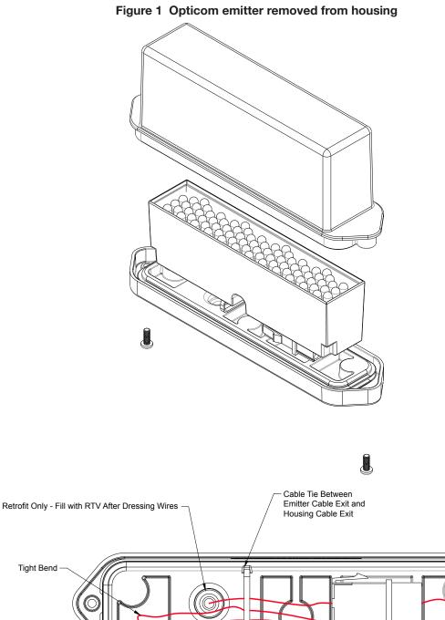
4. After testing the emitter, ensure that the wires are properly dressed. Apply RTV silicone at the location where the cable exits the housing (retrofit only). See Figure 2. Ensure the seal is properly seated on the cap, then slide the housing over the emitter and seat it to the cap.
