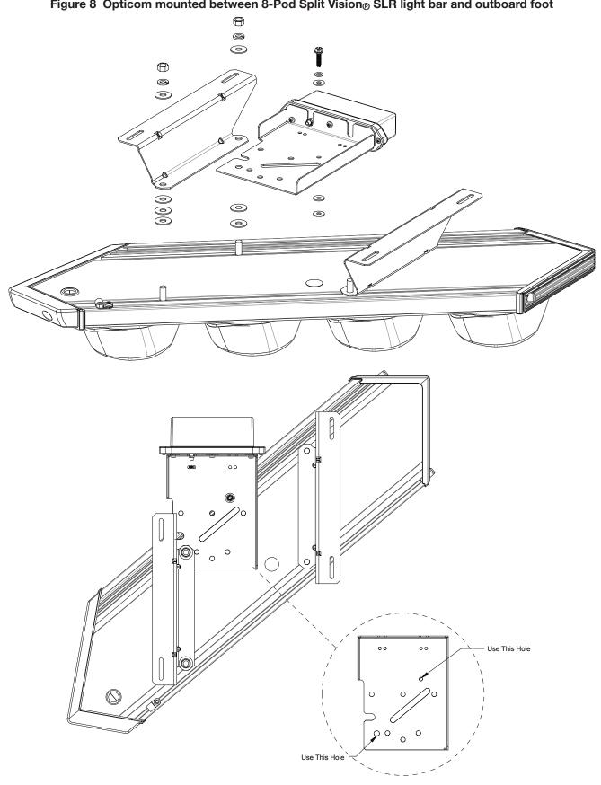
Figure 8 Opticom mounted between 8-Pod Split Vision® SLR light bar and outboard foot
