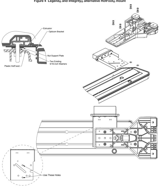
Figure 4 Legend<sub>®</sub> and Integrity<sub>®</sub> alternative HotFoot<sub>®</sub> mount
