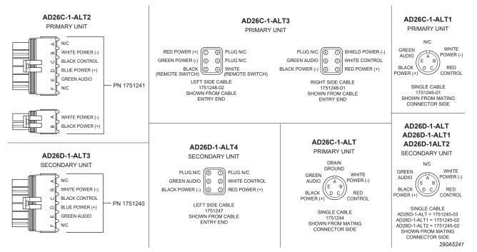
Federal Signal Corporation manufactures several different versions of the Atkinson Dynamics Intercom for Altec Industries Incorporated. Although each of these models are functionally the same as the standard single cable primary (AD26C-1-Z) and secondary (AD26D-1-Z) units, each has its own cable connector(s) and wire colors.
