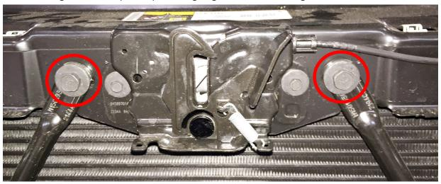
**5.** Using the flat washers as shims between the bracket and angled braces, secure the assembly with bolts removed in Step 4. Relocate or rotate the horn assemblies as necessary. See Figure 2.
