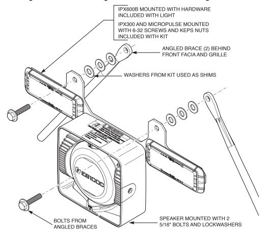
Figure 2 DUR15 mounting bracket secured in front of angled braces
