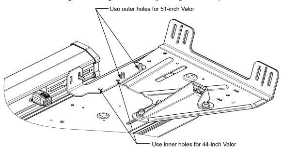
Figure 1 Message Board/Valor (passenger-side view)
