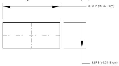
Figure 3 Gasket cut into four equal pieces
