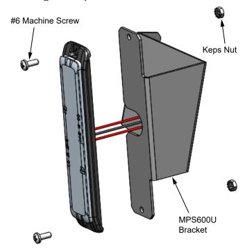
Figure 2 Exploded view of final installation
