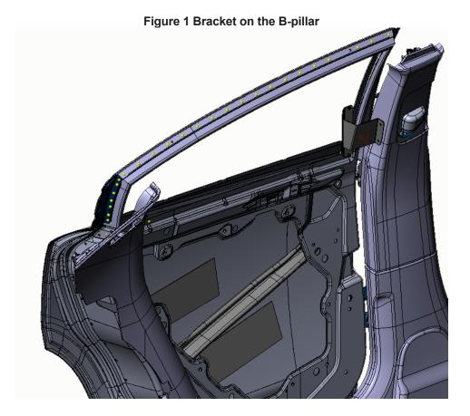
2. Drill a hole for wire routing.
