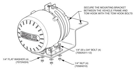
Figure 3 Speaker secured to mounting bracket
