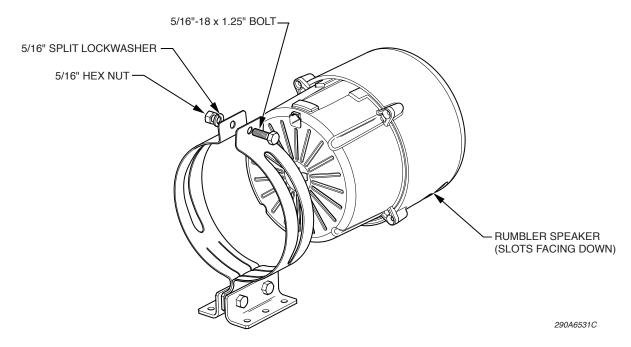
**5.** See Figure 3. Place a speaker and angle bracket assembly on top of a mounting bracket.
