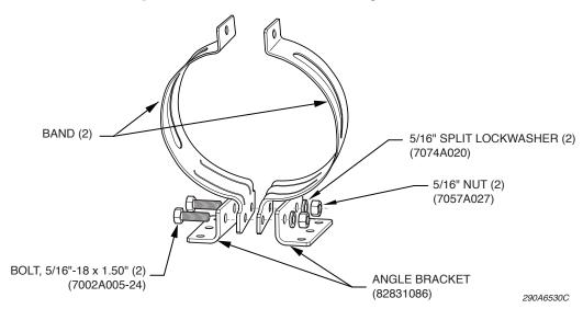
Figure 1 Bands secured between angle brackets
