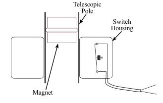
Diagram 1. Pole Down; Magnet Holds Switch Open
