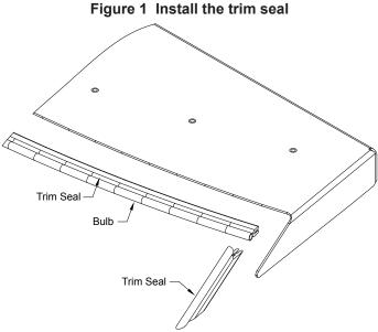
Figure 1 Install the trim seal
