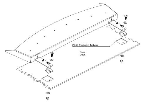
Figure 3 Location of first drilled hole in topside of package tray 2018 Charger
