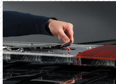
The Allegiant light bar can be serviced while on the rooftop, by removing a single dome and easily disconnecting the ROC board.
