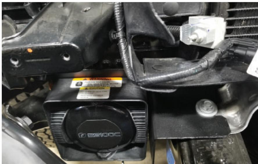
3. Align the bracket so that the slot in the bracket slides underneath the head of the bolt and washer on the vehicle. See Figure 1.
