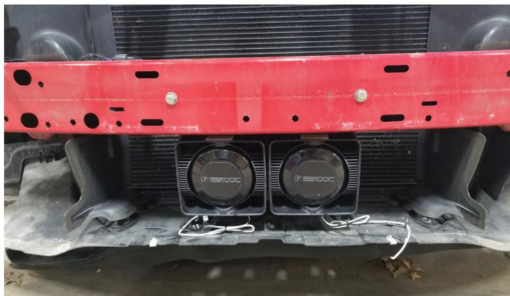
**Figure 2** Exploded view of ESB2-CHGR15 bracket kit installed on Dodge Charger
