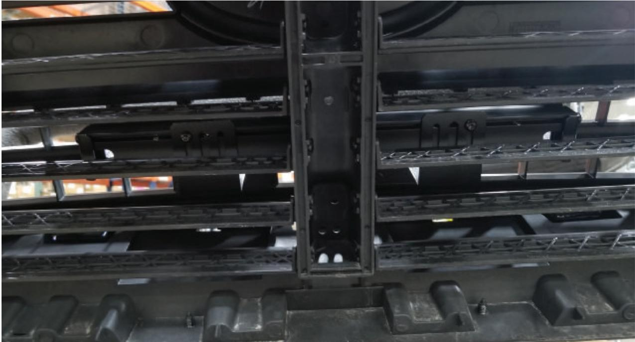
8. Adjust the CN SignalMaster so that it is in the desired position and tighten all hardware. Do not over-tighten.
