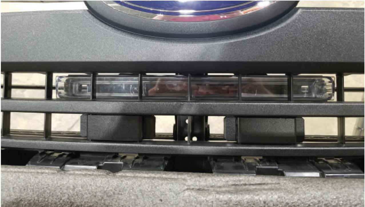
5. Secure the bracket to the grille using a retainer bracket assembly, 2 washers, and 2 elastic stop nuts. Do not tighten hardware.
