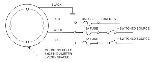
**NOTE:** Use a 3 A fuse to protect all +Vdc connections:
