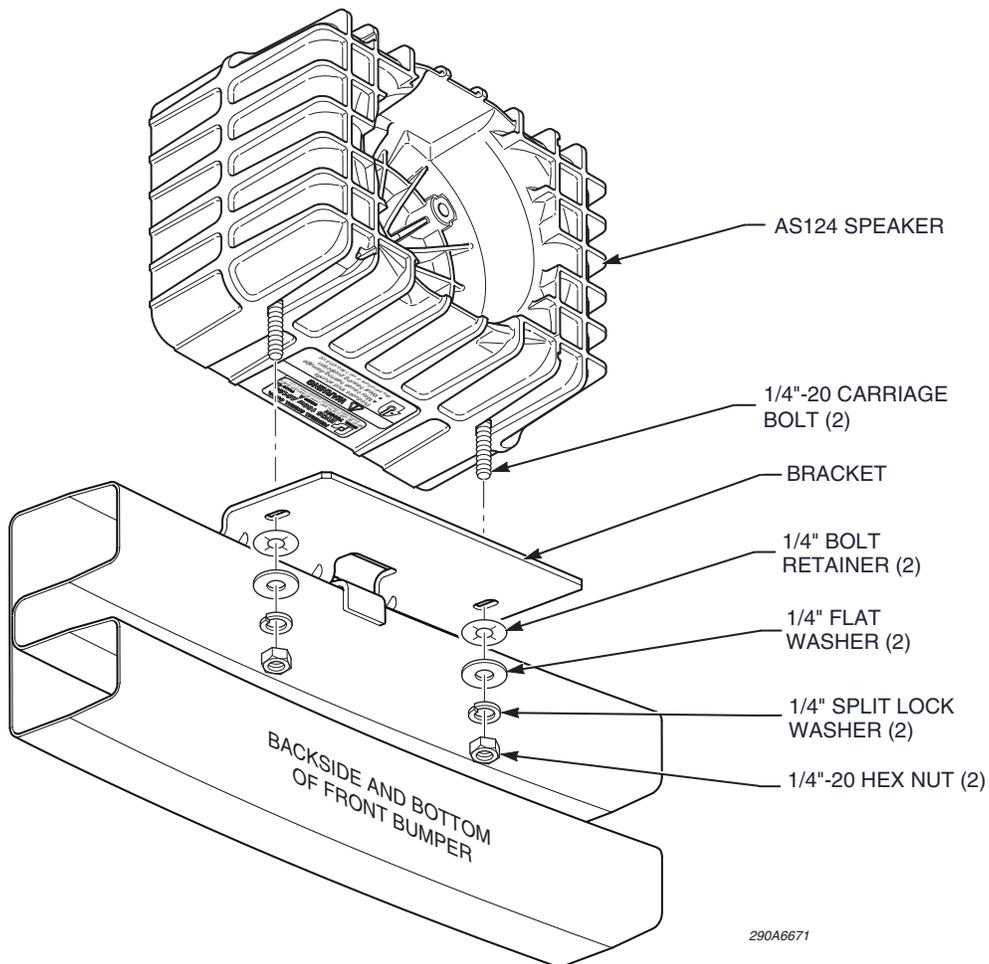
7. Insert the two 1/4" carriage bolts into the bottom of the speaker.
