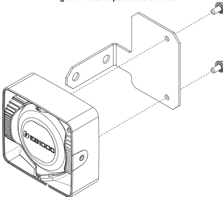
4. Install the speaker/bracket assembly to the driver side tow hook using the two nuts removed in step 2. See Figure 2 for exploded view, and see Figure 3 for the final installation.
