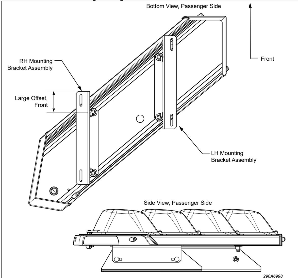
2. Using the mounting brackets as templates, scribe four drill position marks on the mounting surface.
