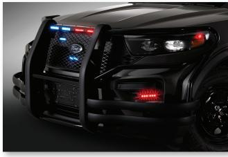
PBX Series Push Bumper, PIT bars, and Wing Wraps are now available for the 2020 Ford Police Interceptor Utility. The PBX Push Bumper Series is designed with maximum safety in mind, and it offers customization for your specific needs while providing the best strength, durability, and protection. All components of the PBX Series are manufactured with heavy duty HRPO steel and engineered to absorb impact and reduce damage to the police car all with officer safety in mind.
