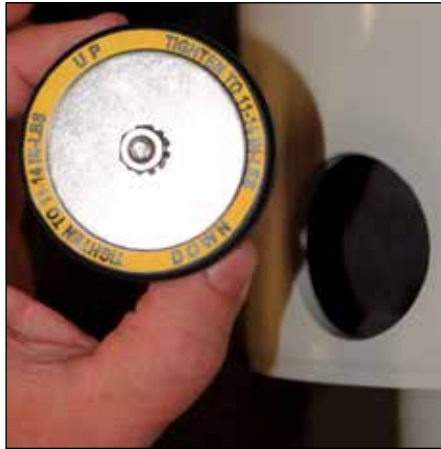
Figure 17 Placing Rubber Plug Over the Access Hole
