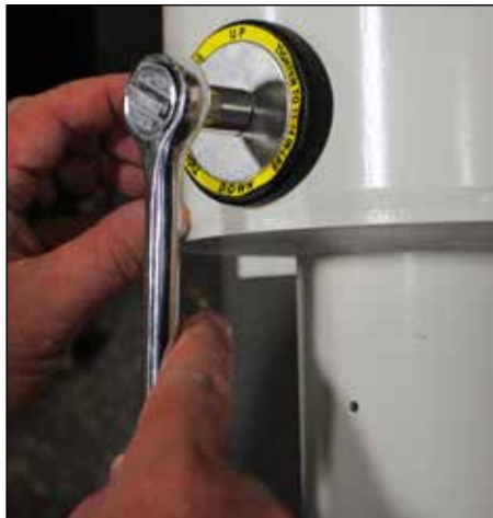
Figure 18 Tightening the Rubber Plug
