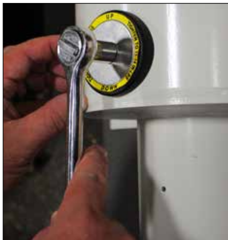
Figure 11 Tightening Rubber Plug
