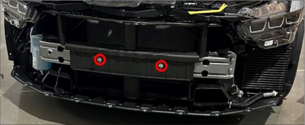
Figure 4 Center bumper bolts to be removed
