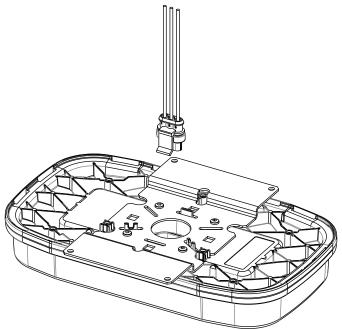
Figure 2 Connecting the Light
