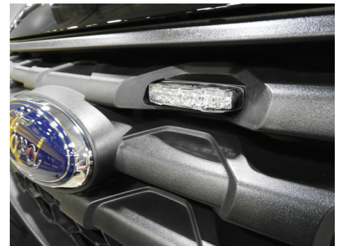
MicroPulse C Series shown mounted in grille
