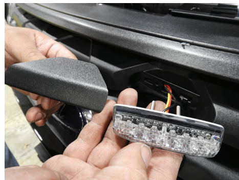
MicroPulse C Series shown with optional stud mount for easy installation
