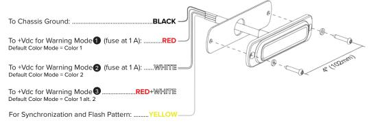
Connect the YELLOW wires of all of the heads together for synchronization. (All heads must be set at the same pattern.)
